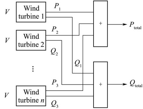
Fig. 6 PQ model of wind farm
