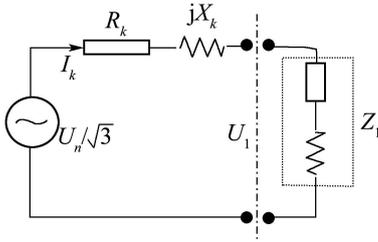
Fig. 1 Equivalent circuit of power grid
