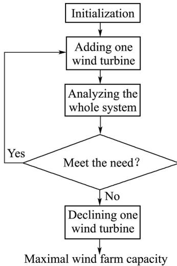
Fig. 11 Calculation of Maximal capacity of wind farm
