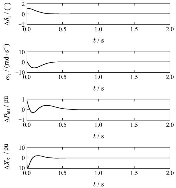
Fig. 3 The state trajectories for the #1 generator with the presented controller in Theorem 1
