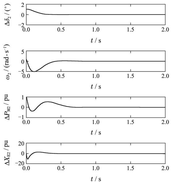
Fig. 4 The state trajectories for the #2 generator with the presented controller in Theorem 1
