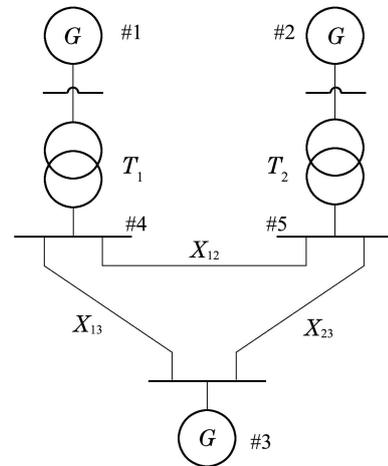
Fig. 2 A two-machine infinite bus example power system
