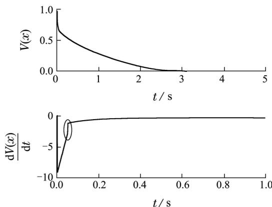
Fig. 4 The evolutions of the quadratic Lyapunov function  $V(x) = x^T P^{\text{Theorem1}} x$  and its time derivative
