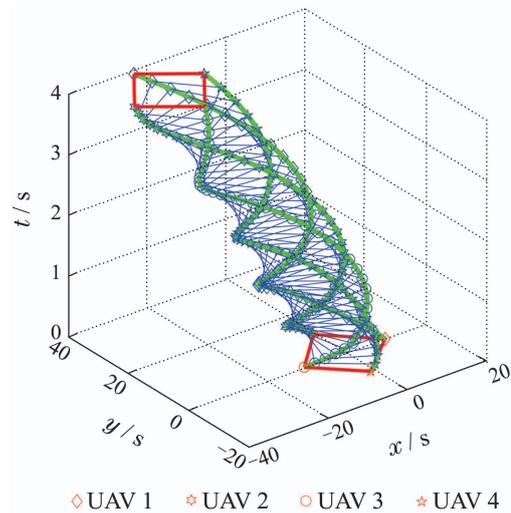
Fig. 4 The formation trajectories of the UAVs
