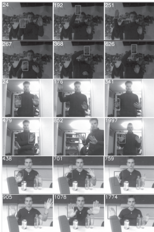
Fig. 4 Three representative challenging sequences used in [13], which captured at different conditions including illumination variation, scale variation, deformation, motion blur, fast motion and background clutters. The object rectangle in each frame obtained by proposed approach is drawn on the image.
