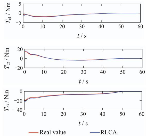
Fig. 8 The real torque value and value computed by SRLSCA in regular polyhedron form
