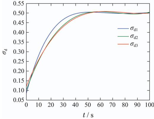
Fig. 2 Desired attitude trajectory  $\sigma_d$  of combined spacecraft
