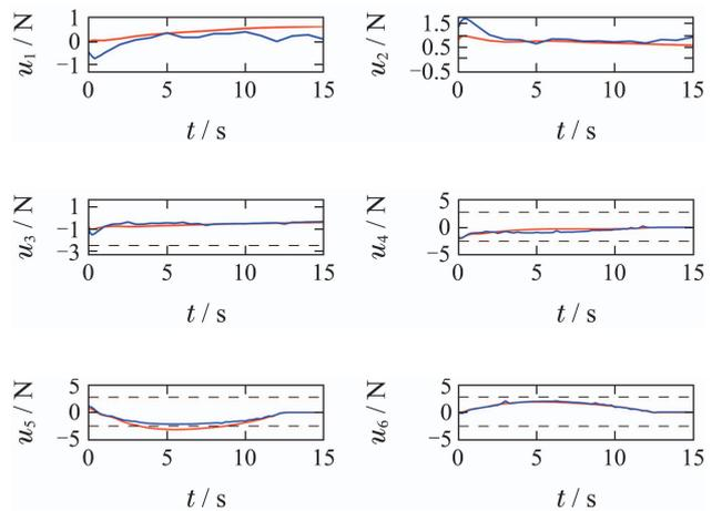
Fig. 9 Results of pseudo-inverse control allocation and SRLSCA in regular polyhedron form
