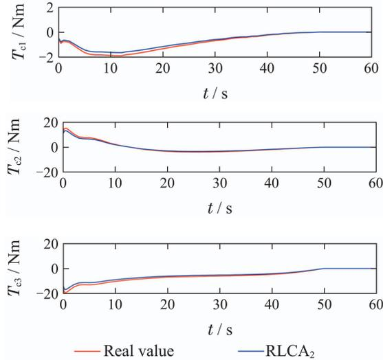
Fig. 10 The real torque value and value computed by SRLSCA in polytopic form
