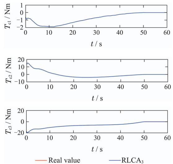
Fig. 12 The real torque value and value computed by SRLSCA with special linear fractional structured uncertainty
