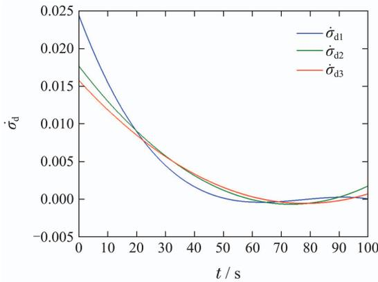
Fig. 3 Desired attitude trajectory  $\dot{\sigma}_d$  of combined spacecraft
