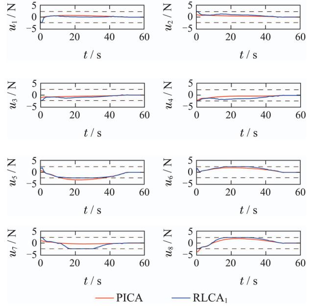
Fig. 7 Results of pseudo-inverse control allocation and SRLSCA in regular polyhedron form
