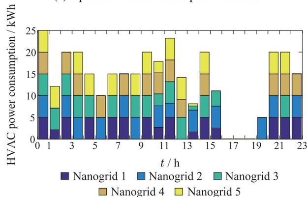
(b) Power consumption of HVAC units in nanogrids
