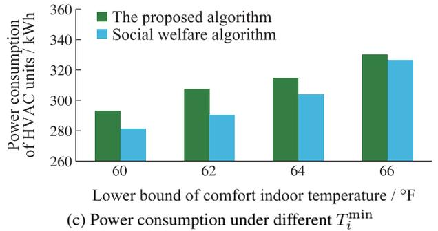
Fig. 6 The impact of  $T_i^{\min}$
