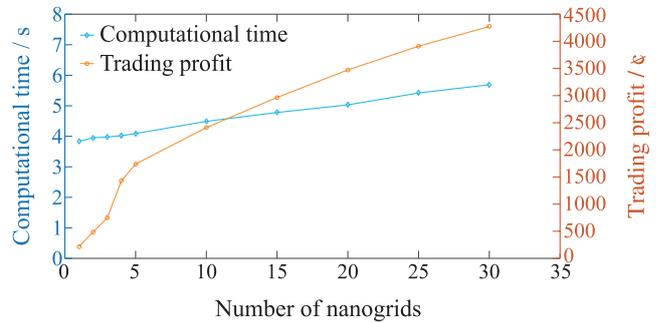
Fig. 11 Optimal results with different number of nanogrids
