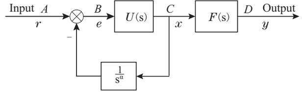
Fig. A1 A sketch diagram of estimation of fractional derivative
