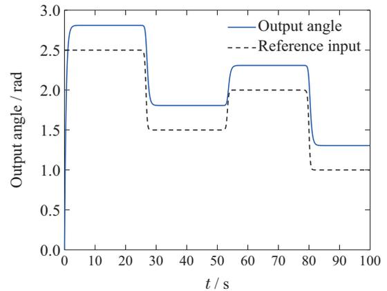
Fig. 13 The position tracking by RRCF
