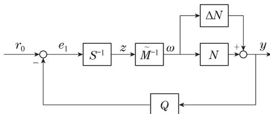
Fig. 8 Tracking control based on dual Bezout
