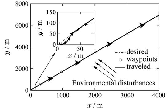
Fig. 4 The practical path generated by guidance law (15) based on the proposed controller
