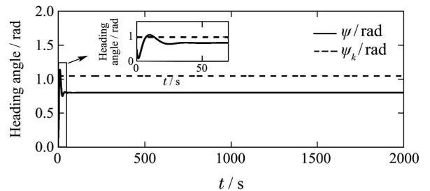
Fig. 5 The practical heading angle with guidance law (8)
