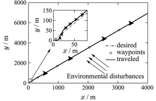
Fig. 3 The practical path generated by guidance law (8) based on the proposed controller
