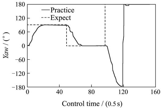
(a) The curve of low-speed directional control
