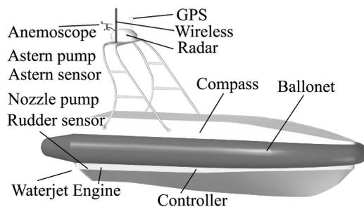
Fig. 1 The equipment of the USV system
