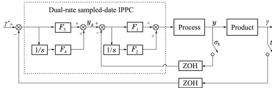
Fig. 2 Dual-rate sampled-data IPPC scheme
