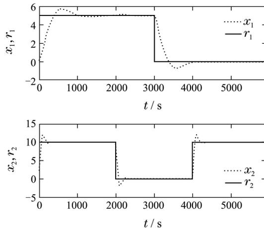
Fig. 3 Outer loop tracking performance for square waves
