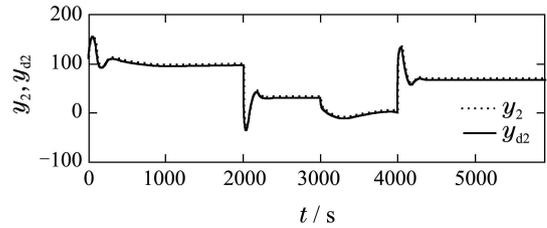
Fig. 4 Inner loop tracking performance for square waves
