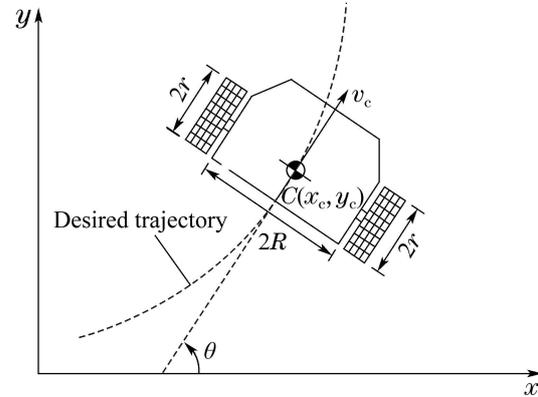
Fig. 1 The nonholonomic wheeled mobile robot
