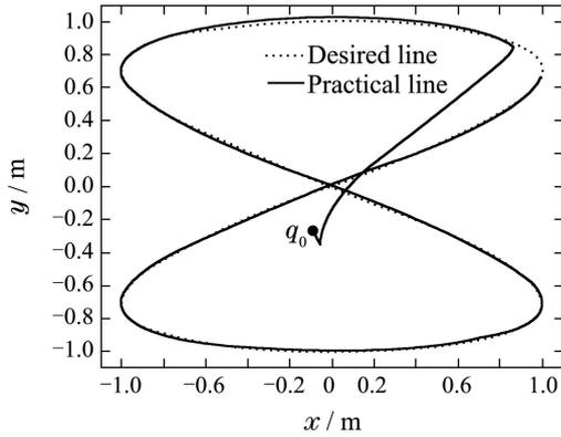
Fig. 3 Tracking for an eight-shaped trajectory
