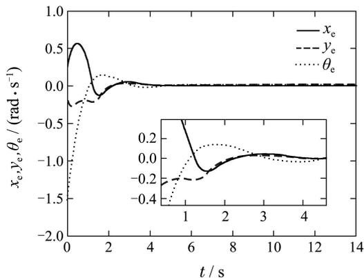
Fig. 5 Posture errors of the mobile robot
