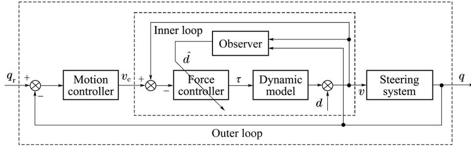
Fig. 2 Double closed-loop control structure
