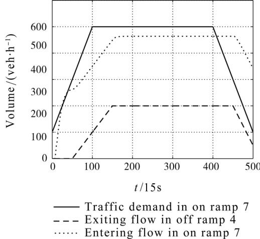
Fig. 3 Traffic demand in on-ramp 7, entering flow in on-ramp 7, and unknown exiting flow in off-ramp 4
