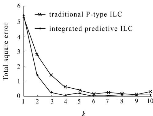
Fig. 2 Tracking performance of IPILC compared with the traditional ILC
