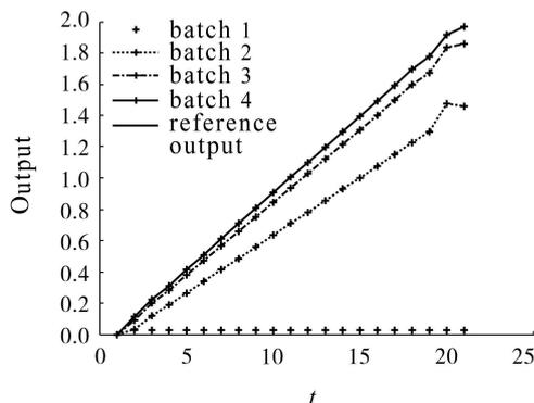
Fig. 1 Tracking performance of the system output at different time steps and batches under IPILC
