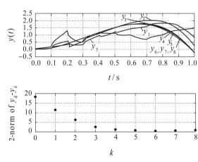
Fig. 2 The system outputs  $y_k(t)$  and the 2-norms of  $e_k(t)$  for different iterations, where  $k \in \{0, 1, 2, \dots, 8\}$  and  $\xi = \frac{2}{5}$ .
