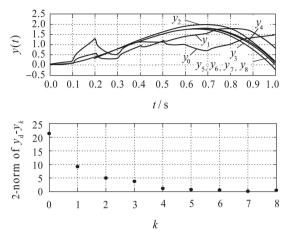
Fig. 1 The system outputs  $y_k(t)$  and the 2-norms of  $e_k(t)$  for different iterations, where  $k \in \{0, 1, 2, \cdots, 8\}$  and  $\xi = \frac{1}{2}$ .
