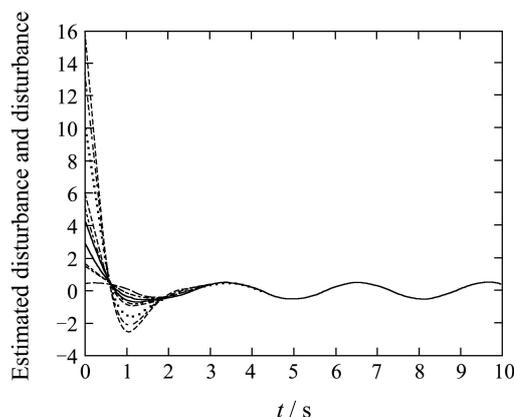
Fig. 3 Disturbance estimated by the disturbance observer
